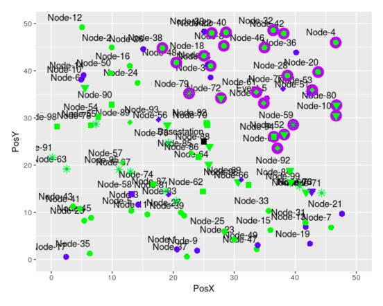
Fig. 17 Example of the EC-CKN network. Green means active, blue means sleep, a purple ring means the node has sensed an event, and a purple circle means an event.
