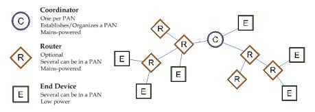
Fig. 9 Zigbee mesh network layout
