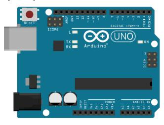
Fig. 8 Arduino UNO board
