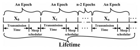
Fig. 3 Network lifetime broken up into epochs<sup>6</sup>
